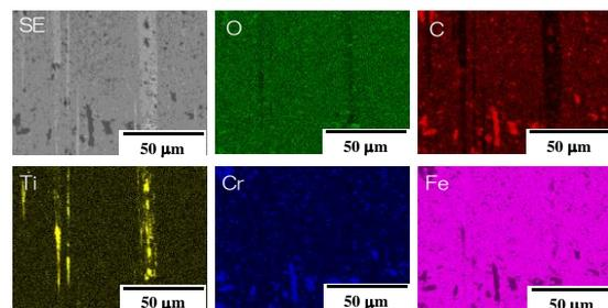
Figure 2: SEM-EDX analyses at the center on the contact interface of cs-AISI420J2 punch to titanium work. a) SEM image on carbon and titanium oxide layers, and b) element mapping.
