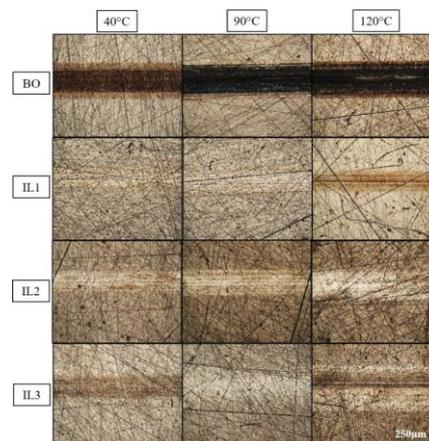
Figure 1: Confocal microscopy image of wear tracks on steel substrates after SRV tests under an additive-free base oil (BO) and IL's 1-3 at distinct temperatures of 40, 90 and 120 °C.
