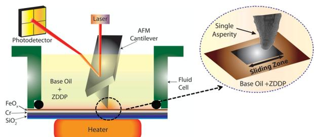
Fig. 1: Schematic of setup used for tribofilm formation.
