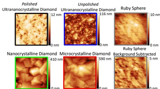
Figure 1: 2.5- $\mu\text{m}$  AFM scans of diamond coatings. [2]
