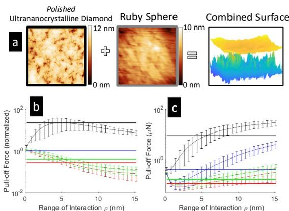
Figure 2: Experimental results (horizontal lines) were fit by integrating an interaction potential over measured topography. (Colors match Fig. 1.) Best-fit values were extracted for work of adhesion and interaction range. [2]
