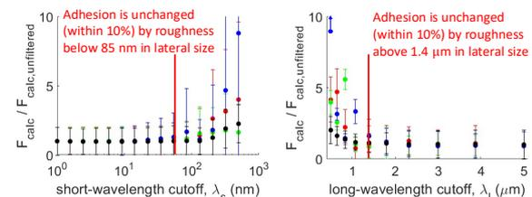
Figure 3: For each substrate, the pull-off force  $F_{\text{calc}}$  was calculated with all scales of roughness included, and with a short- or long-wavelength cutoff. (Colors match Fig. 1.) The fractional difference in pull-off force indicates the relative contribution of the filtered scales. [2]
