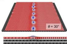
Figure 1: A corrugated graphene grain boundary with misfit angle of  $30^\circ$  supported by a pristine graphene bilayer. The lower layer serves as a rigid support during the simulation. Periodic boundary conditions are applied in the lateral directions.
