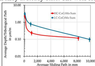
Figure 1: Ratio of the Average Depth of the Wear Scar per Sliding Path in  $\mu\text{m}/\text{m}$ .
