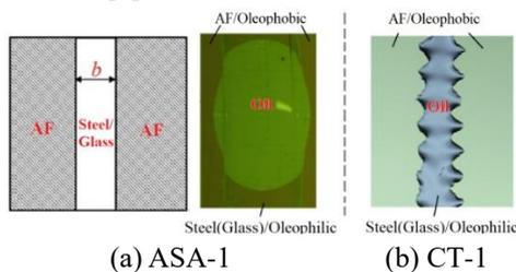
Figure 1: Fabricated oleophilic lubrication track with side wettability step
