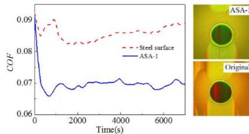
Figure 2:  $COF$  for a steel ball (9.5mm in diameter) loaded against treated and untreated steel plates, PAO4, 10 N, 0.5  $\mu\text{L}$ , sliding frequency = 8 Hz.
