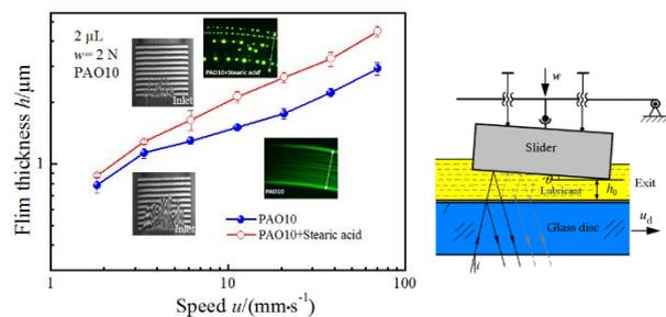
Figure 3: Film thickness in slider-on-disc contact for PAO10 with/without stearic acid, slider size: 4mm×4mm, slider inclination:  $\theta=5.89 \times 10^{-4}$
