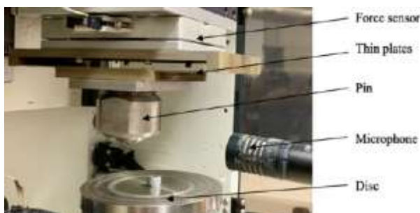
Figure 1: Pin-on-disc squeal test rig.
