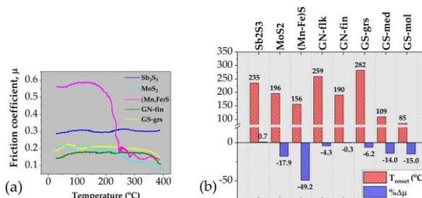
Figure 1: (a) Friction coefficient vs. temperature. (b) Friction decreasing temperature ( $T_{\text{onset}}$ ) and friction variation ( $\% \Delta \mu$ )
