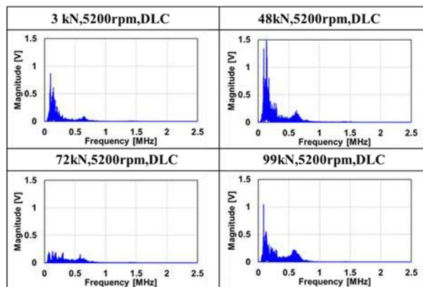
Fig.2 AE analysis results of DLC coating shaft
