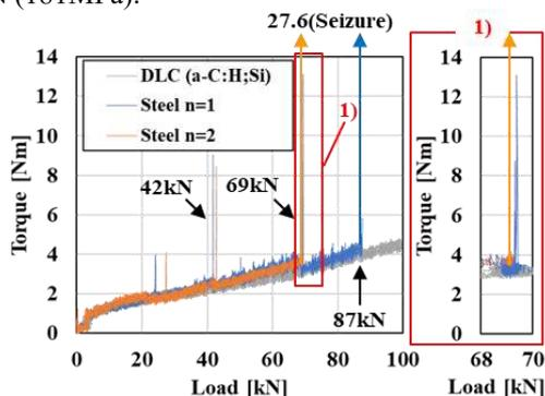
Fig.1 Torque spikes and seizure with or without DLC coating
