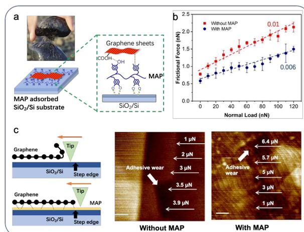
Figure 1: (a) Schematic diagram of Gr/MAP film; (b) friction force as a function of the applied normal load for AFM Si tip sliding on graphene with and without MAP; (c) wear-resistance of graphene at the step edge.
