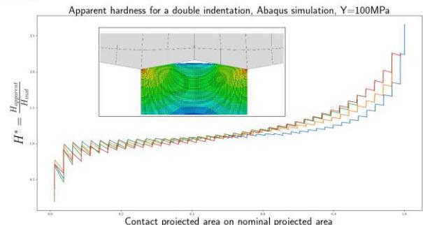
Figure 2: Apparent hardness normalized by material hardness plotted against normalized contact area during double indentation loading.
