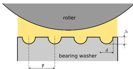
Figure 1: A schematic of the profile of the laser textured surface in a lubricated contact condition.
