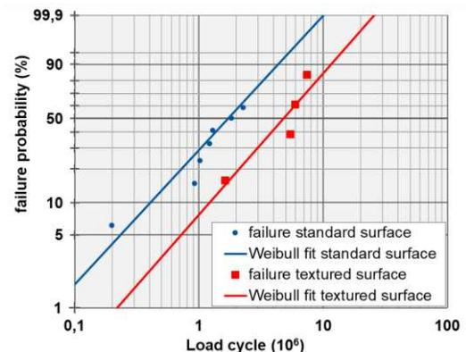
Figure 2: Weibull distribution of the fatigue tests of the reference and the Cross30 laser textured thrust ball bearings.
