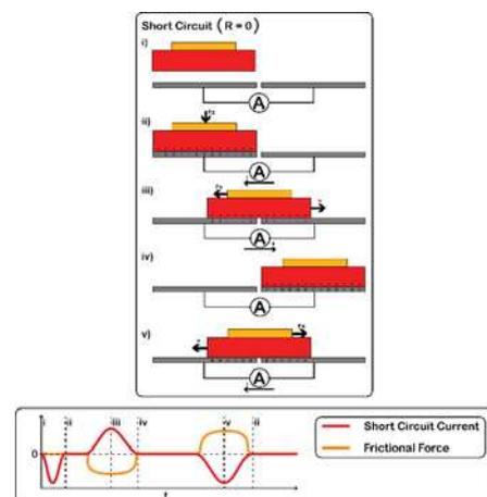
Fig.1 – Schematic representation of the F-TENG contact with the electrometer configured to measure short-circuit current.
