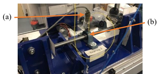
Figure 1: Test rig containing a conventional electronic accelerometer (a) and an FBG sensor (b).
