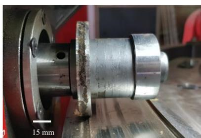
Figure 1: Roller-Ring contact reality with dead leaves on the tribometer “*Triboring*”
