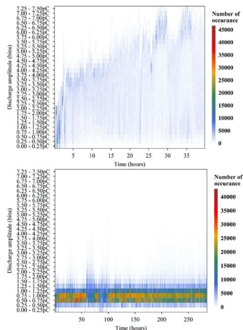
Fig. 2. Charges detected by ES for a WEC failed test (upper) and non-failure test (lower).
