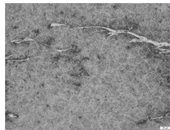
Fig. 1. Subsurface optical image showing WECs created in one of the TE74 rollers.
