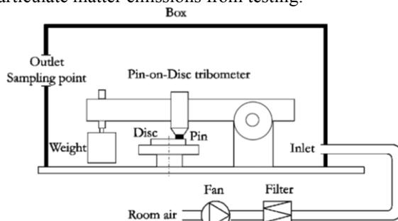
Figure 1: Schematic of the test equipment.
