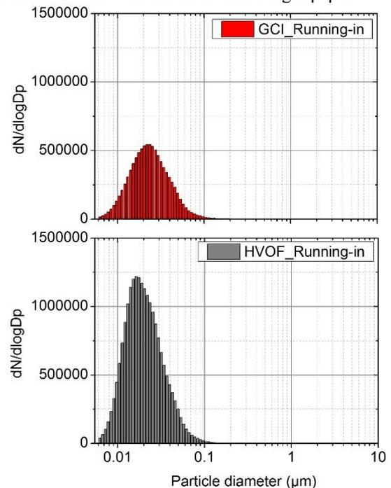
Figure 2: Size distribution of the ultrafine particles in the running-in period.
