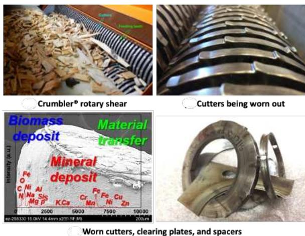
Figure 1: Crumbler® rotary shear biomass comminution system and its worn components.
