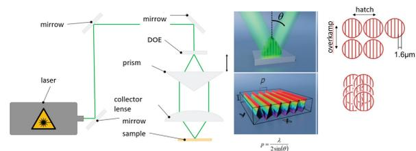
Figure 1: Scheme of the DLIP technique to perform structures on the surface
