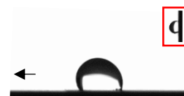
Figure 3: Image of a water droplet on the stainless steel 316L surface presenting micrometric squares as a texture as shown in Figure 1. The surface is tilted by 90° in the direction of the arrow on the picture. For better visualization of the reader, the image in the red box represents how the surface is during the experiment.
