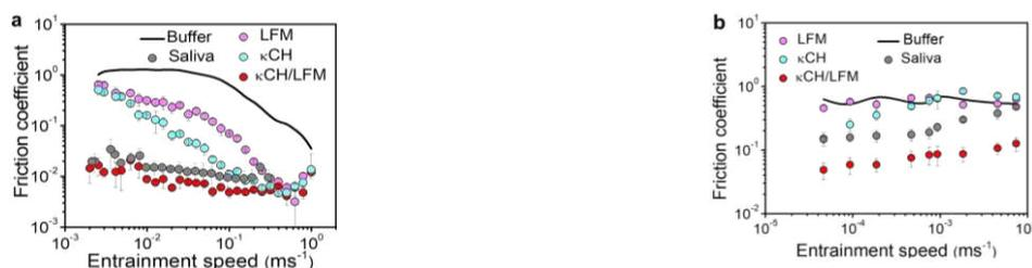
Figure 2. The friction coefficient results for LFM,  $\kappa$ CH, LFM-doped  $\kappa$ CH and real human saliva on elastomeric surfaces using a) MTM and b) a modified rheo-tribometer and tongue mimicked surfaces.
