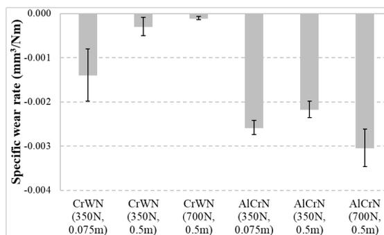
Figure 1: Specific wear rate for CrWN and AlCrN coatings sliding against Al-Si coated 22MnB5 steel.
