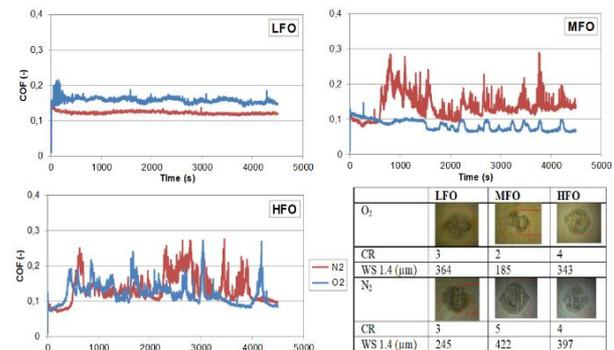
Figure 1: COF versus time graphs and ball wear scars for fuel oils at 100 °C in air and in nitrogen atmosphere.
