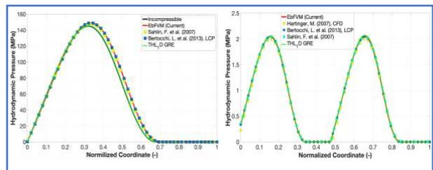
Figure 2: Results for single and double parabolic sliding bearings.  $THL_1D GRE$  is the current framework.
