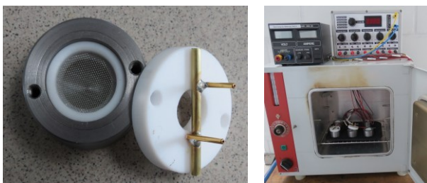
Figure 1: Test chamber and current feed apparatus.
