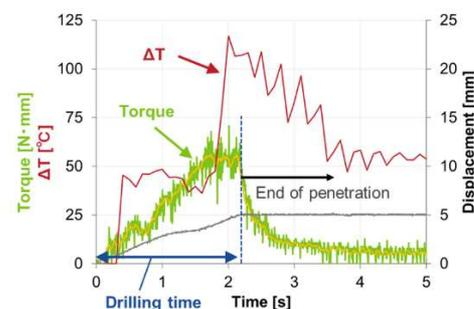
Figure 1: Typical curves of drilling properties in PU50
