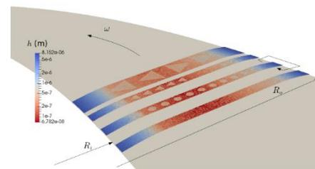
Figure 1 Configuration of the problem and example of film thickness results.
