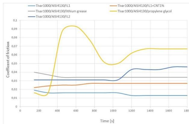
Figure 1: Selected time-dependent changes in the coefficient of friction for Tivar 1000 polyethylene – the AISI 4130 pair and various types of lubricants.
