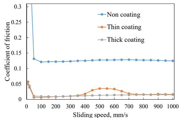
Figure 1: Variations in friction coefficient at different sliding speeds for three discs
