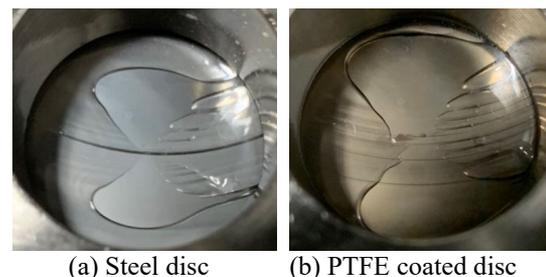
Figure 2: Comparison in meniscus pattern between steel disc and PTFE film coated disc.
