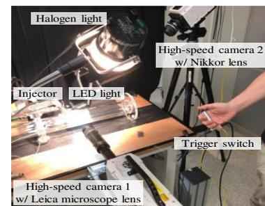
Figure 1: Test set up for visualization experiment.
