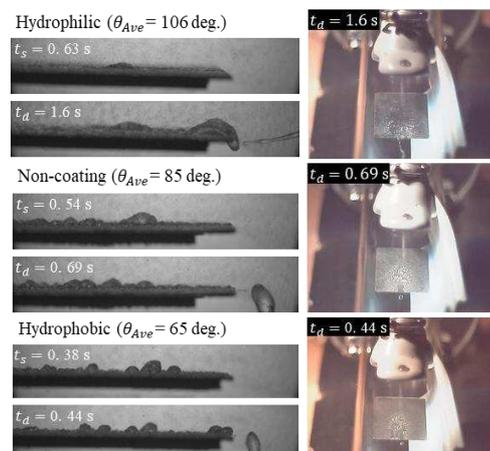
Figure 2: Visualization results of liquid film behavior (Visualization speed: 5000 fps, Exposure time 0.2μs).
