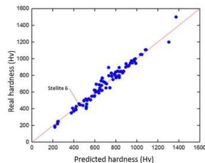
Fig.1 Real hardness as a function of predicted hardness calculated from Gaussian process model.
