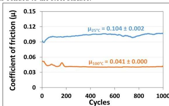
Figure 1: Friction curves of PAO 4 + PFM at 25°C (in blue) and 100°C (in orange). Tests are carry out on reciprocating tribometer (1 GPa, 0.003m/s) and values of friction coefficient ( $\mu$ ) are averaged between 400 and 1000 cycles.
