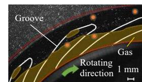
(a) Flow visualization at 2,000rpm
