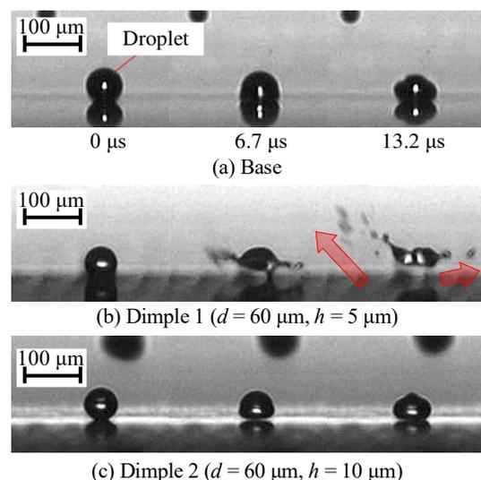
Figure 3: Visualization results for each test piece.
