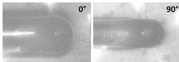
Figure 2: Pictures of scratches on oriented iPP depending on the sliding direction (0°= parallel to the draw axis) .
