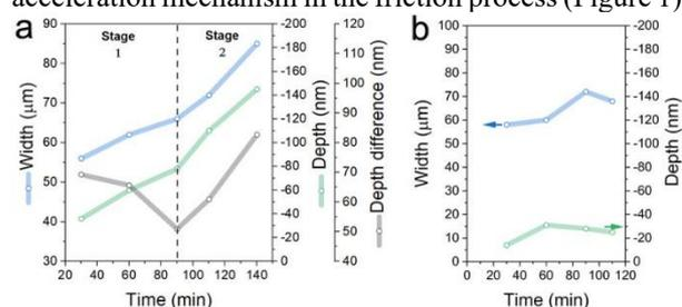
Figure 1: Evolution of width and depth of wear scars with test time under oil-lubricated condition (a, PAO+MoDTC; b, PAO).
