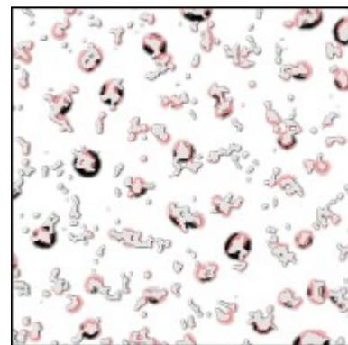
Figure 1: Crack nucleation sites (black), plastic zones (red) and micro-contacts (gray) for the  $J_2$  plasticity model.
