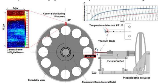
Figure 1: Schematization of the test rig and its instrumentation.
