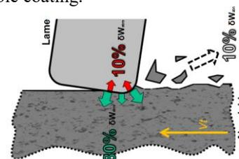
Figure 2: Result of the energy balance.
