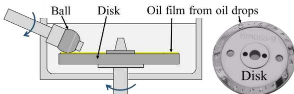
Figure 1: MTM2 for loss-of-lubrication tests
