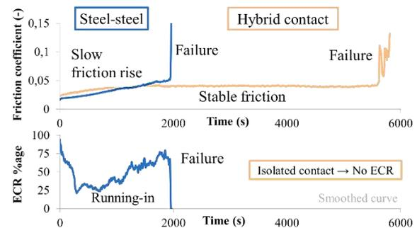
Figure 2: Friction and ECR curves for 2 loss-of-lubrication tests (steel-steel contact and hybrid contact)
