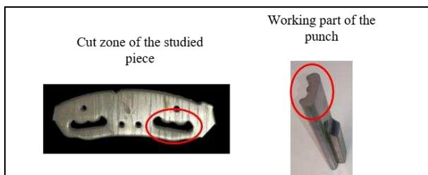
Figure 1: Geometries of the blanked parts and the corresponding punch.
