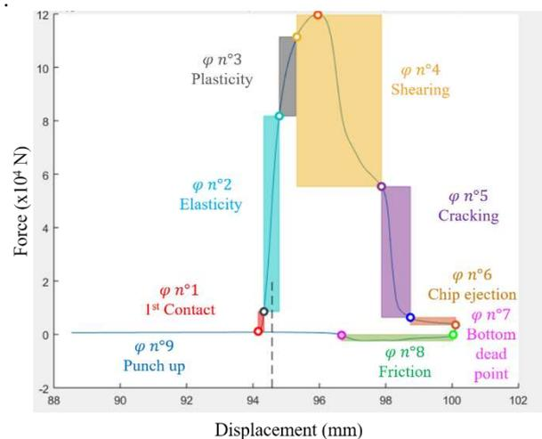
Figure 2: Identifying the force/displacement cycle of the punch during a fine blanking operation
