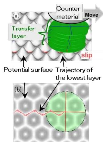
Figure 1: Thermal escape motion which is found by coarse-grained molecular simulation [3].
