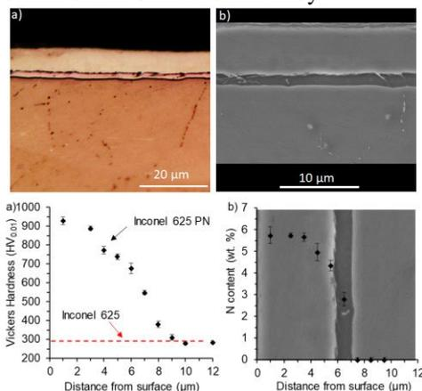
Fig. 2 Microstructure, microhardness and nitrogen concentration profiles of Inconel PN 625.
