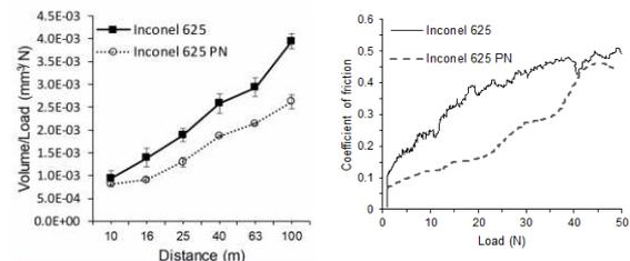
Fig. 4 Micro-abrasive response of PN Inconel 625 in microabrasion and linear scratch tests.
