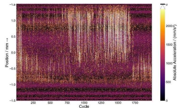
Figure 2 Triboscopic image of the absolute value of acceleration demonstrating the detection of stick-slip behavior
