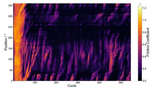
Figure 1 Triboscopic image of rotational experiment of ta-C-steel contact at  $10^{-1}$  mbar demonstrating two features: running-in (“Persistent in cycle”) and dragged-along debris from abrasion (“Random”)
