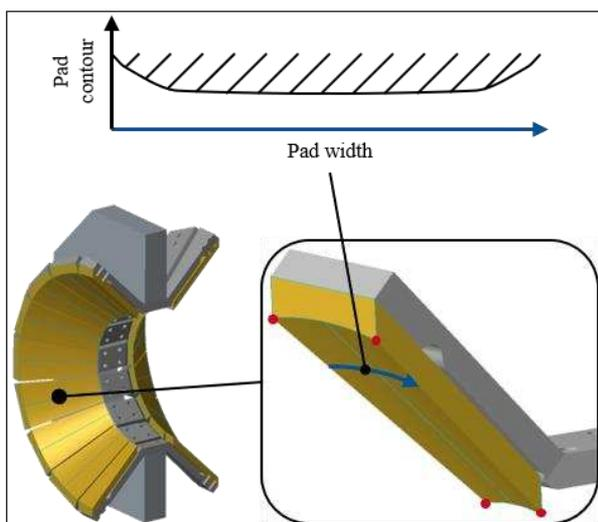
Figure 1: CAD model of FlexPad demonstrator (bottom left). Detail of double flexible pad mount with attached sliding pad (bottom right). Possible pad contour (top).
