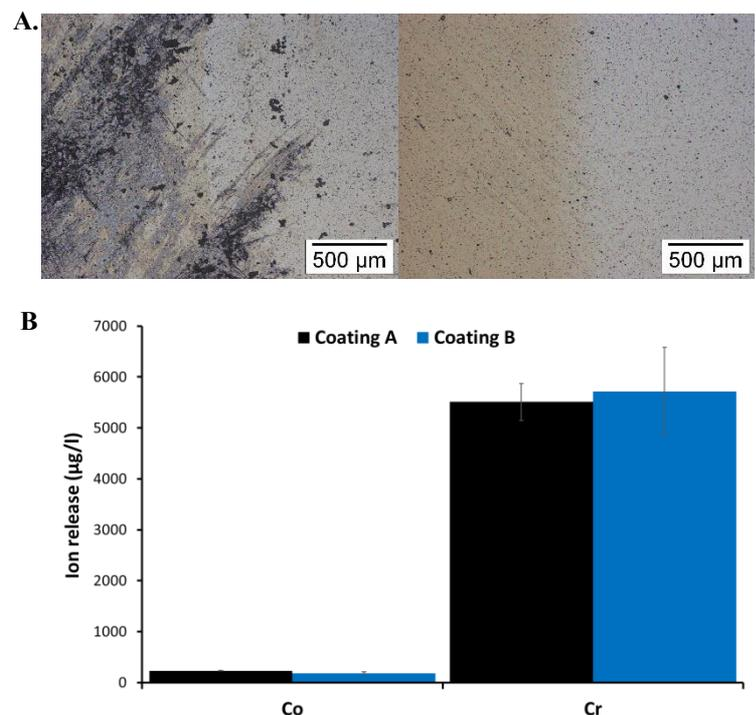
Figure 1. (A) Microscopy images of Coating A (left) and Coating B (right) on CoCrMo disks after 1 million cycle wear tests. The images show one representative test per type. (B) Cobalt and chromium ion release in the bovine calf serum after 1 million cycle. The serum was collected from each station and analysed at every change. The data represent the average of 5 tests per type over 1 million cycle wear tests.
