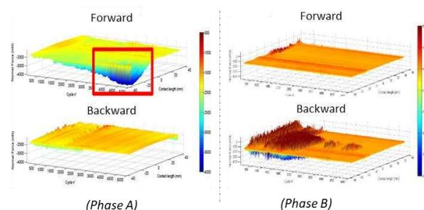
Figure 1: Variation in the normal load at the pad/disc interface, in vacuum. Material: commercial Duroïd 5813
