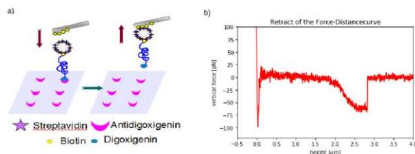
Figure 1: a) Sketch of cantilever preparation, using the adhesive interaction between biotin-functionalised DNA molecule and streptavidin-coated micrometer bead b) Exemplary force-distance curve with typical stretching properties of single DNA molecules and a rupture event
