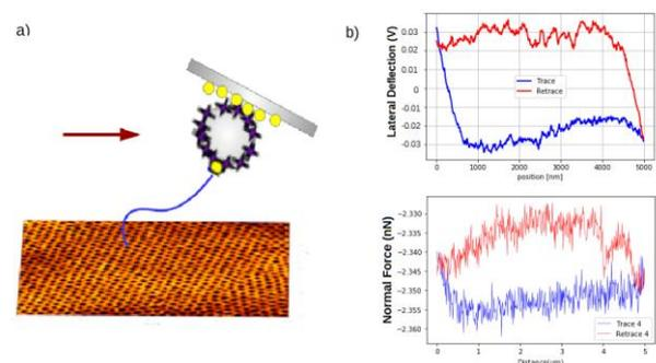
Figure 2: (a) Sketch of friction force measurement with DNA-functionalized cantilever on the porous membrane. (b) Lateral and vertical deflection of a friction loop for a sliding distance of 5  $\mu\text{m}$  618 nm above the membrane surface.
