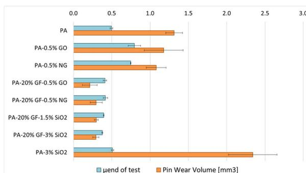
Figure 1: The friction coefficient and the wear volume in the end of the pin-on-disc tests of the polymer composites.
