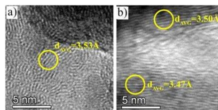
Figure 1: Lamellar distance ( $d_{002}$ ) of SiC derived graphite (a)  $\alpha$  SiC (b)  $\beta$  SiC.
