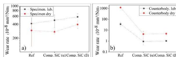
Figure 2: Wear rate in dry and lubricated condition a) Specimen b) Counterbody.
